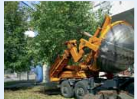
During the rebuilding of the Nuremberg stadium 20 old lime trees were saved. The trees were uprooted with special machinery and later replanted adjacent to the stadium following completion of building work.
